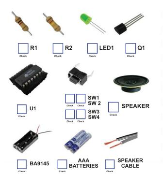
The HK625 Integrated Circuit can produce 4 sound effects, fire, police and ambulance siren as well as raygun fire. This is accomplished by pressing the appropriate PB switch on the circuit board. When a sound is activated an LED also flashes. The audio output from the integrated circuit is amplified by the BC639 transistor circuit to provide sufficient volume at the speaker. The kit is powered from a 3V 2AA battery pack.
